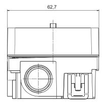
When replacing LAE10 and LFE10 with LFS1, adapter KF8896 ensures that the height can be adjusted mechanically and that the terminals are assigned correctly.
