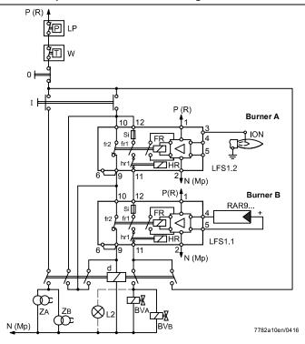
With this type of supervision, too, the burner can be started only if the flame detector test or flame simulation test has been successful. This means that **neither** of the 2 flame safeguards may detect a flame signal during burner off times. When the burner is started up, the detector test will automatically be interrupted. When button (I) is pressed, relay (d) is energized via circuit path 9...10 of the flame relays, which is still closed, thus switching on the ignition of both burners.
