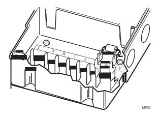
Fig. 13. Attaching a shunt resistor to TRADELINE motors.
