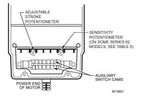
Fig. 12. Stroke adjustments setup.
