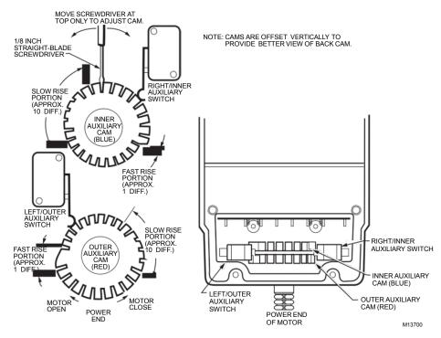
Fig. 14. Auxiliary switch adjustment.
