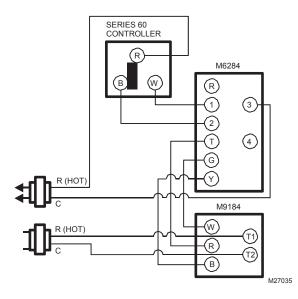
Fig. 10. Series 60 and Series 90 in Slaving Application
