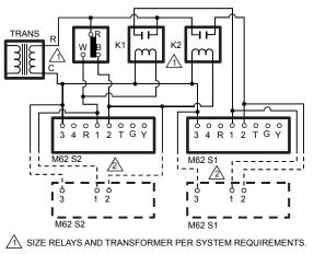
ADDITIONAL SERIES 2 OR SERIES 1 MOTORS CAN BE ADDED IN PARALLEL. DO NOT MIX SERIES 1 AND SERIES 2 IN THE SAME LINE. ONLY WIRE SERIES 1 WITH SERIES 1 AND SERIES 2 WITH SERIES 2 IN PARALLEL. M27044
