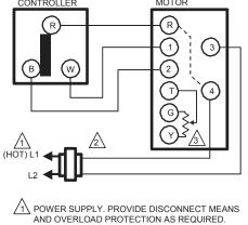
TRANSFORMER MAY BE INTERNAL OR EXTERNAL TO MOTOR.
